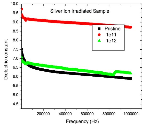
Fig. 1: Dielectric spectrum of Poly vinylidene chloride samples irradiated with different fluences of silver ions
