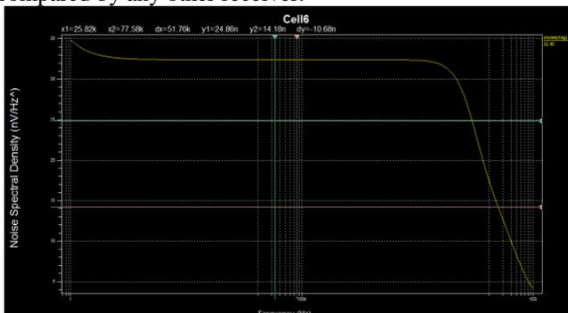
Fig. 8: output referred noise of US receiver
