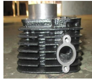
Fig. 4: Photograph of cylinder block The newly developed SPM is shown in fig.4. below
