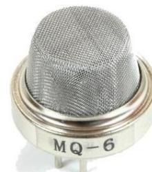
Fig. 2: MQ-6 sensor
