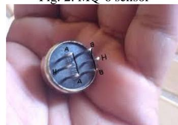
Fig. 3: Pin description of the sensor
