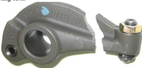
Fig. 4: Failure of a rocker arm at neck
