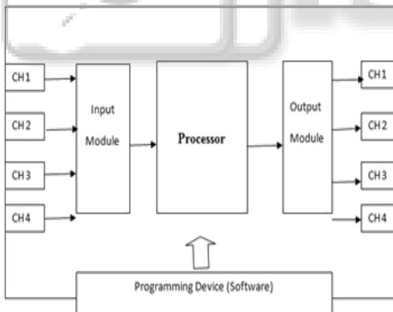
Fig. 1: PLC Architecture
