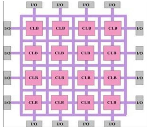
Fig. 2: Overview of FPGA Architecture
