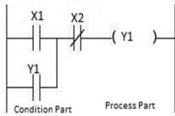
Fig. 3: Overview of Ladder Diagram
