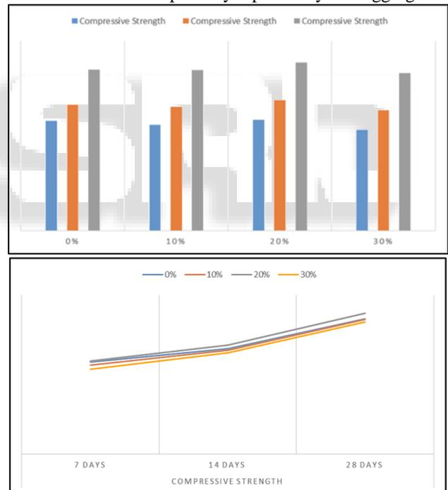
Fig. (1) & (2): Compressive Strength of glass powder concrete when cement is partially replaced
