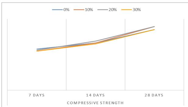
Fig. (3) & (4): Compressive Strength of glass powder concrete when fine aggregate is partially replaced
