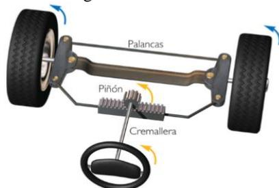
Fig. 1: Rack & Pinion
