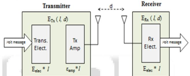
Fig. 2: General radio transmitter and receiver model
