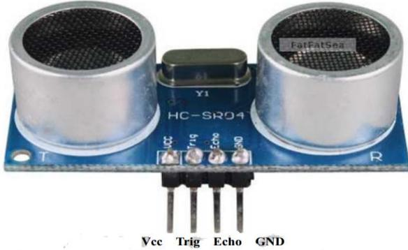
Fig. 2: Ultrasonic Ranging Module HC - SR04
