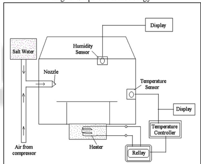
Fig. 3: Block Diagram of Salt Spray Humidifier
