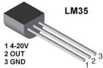
Fig. 2: LM35 temperature sensor
