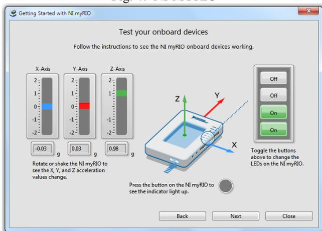
Fig. 5: 3 axis measurement by using NI-MYRIO
