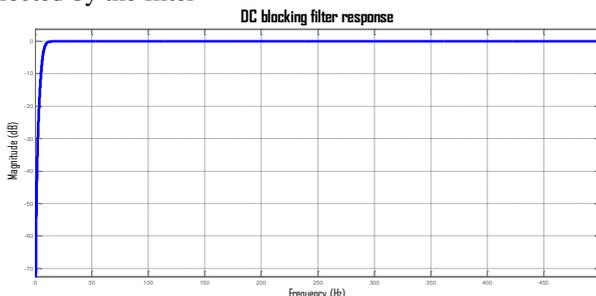
Fig. 2: DC blocking filter response
