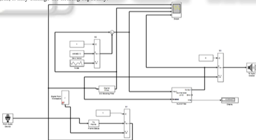
Fig. 1: Simulink block model for Noise cancellation in DHA
