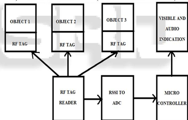
Fig. 1: Schematic of the wearable device
