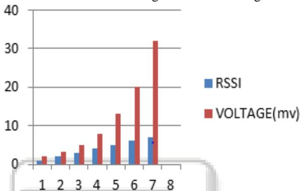
Fig. 2: RSSI level vs Voltages
