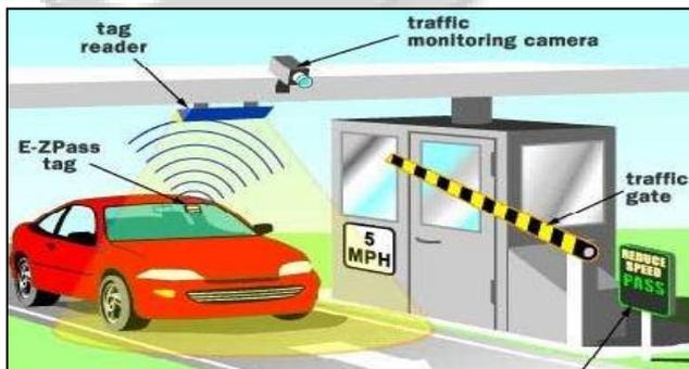
Fig. 1: Demo of WSN Based RFID System
