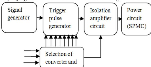
Fig. 5: Block diagram for selection of converter
