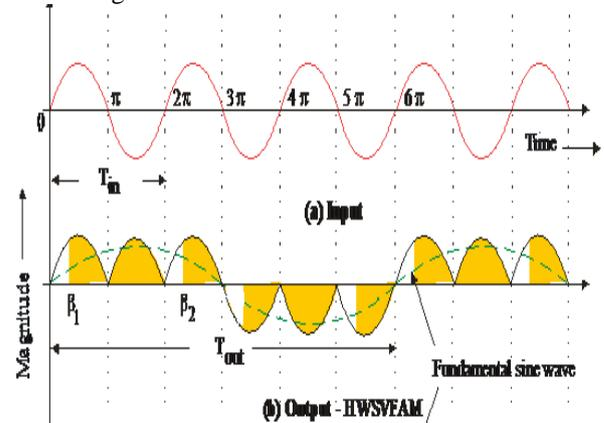
Fig. 8: Half wave symmetry variable firing angle schme
