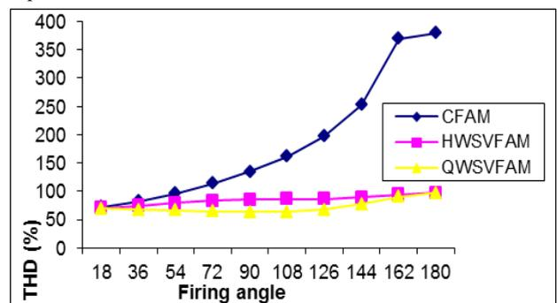
Fig. 14: Comparison of THD with Firing Angle between Proposed Methods and CFAM
