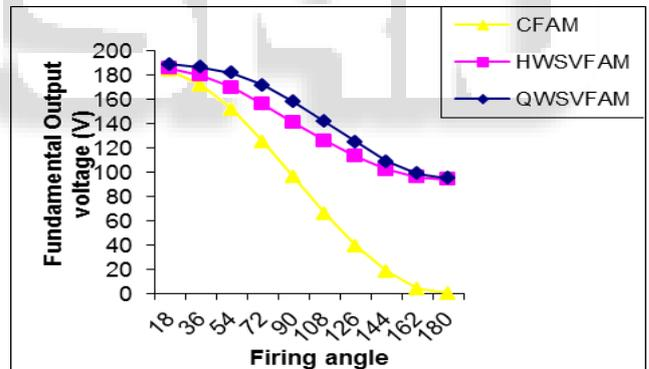
Fig. 13: Comparison of Fundamental Voltage with Firing Angle between Proposed Methods and CFAM
