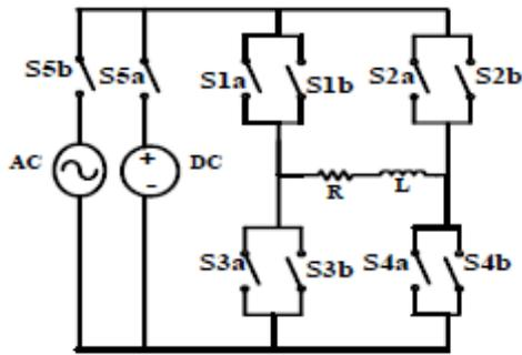
Fig. 7: Generalized single phase matrix converter
