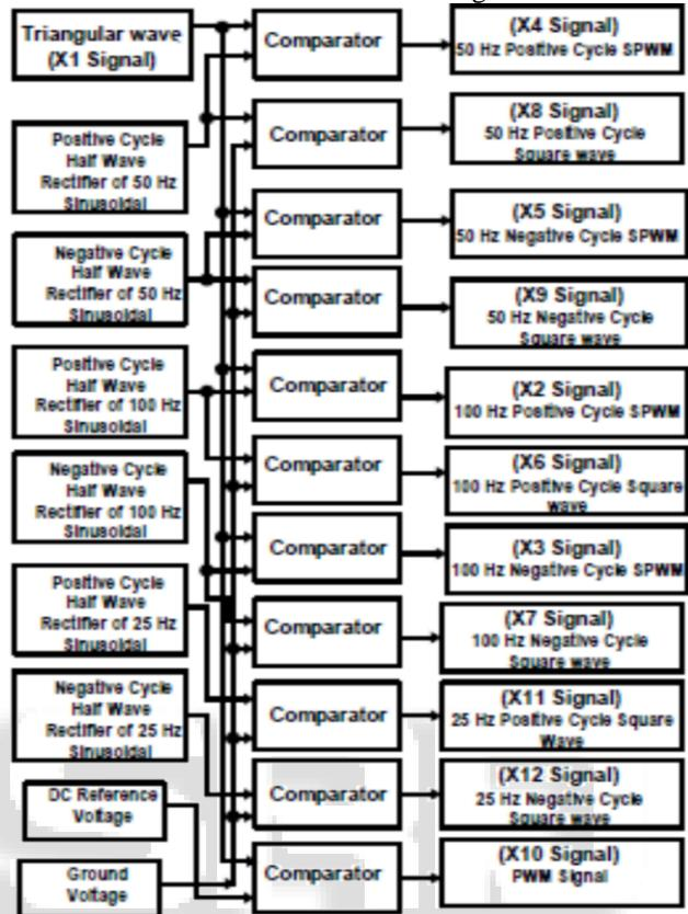
Fig. 6: Basic signal generator block
