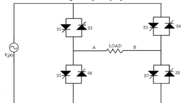
Fig. 1: single phase matrix converter topology
