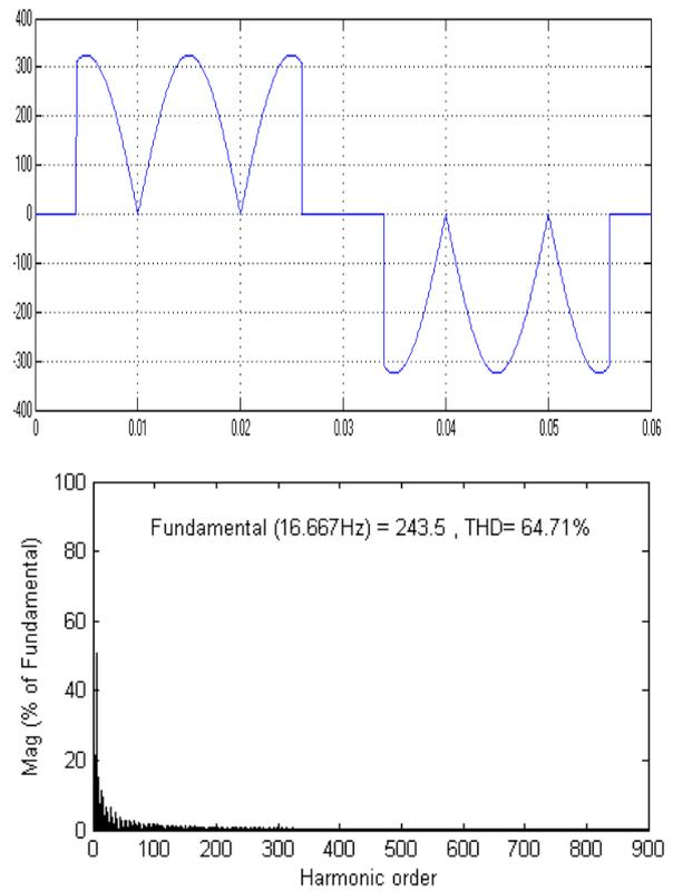
Fig. 12: Quarter Wave Symmetry Variable Firing Angle Method
