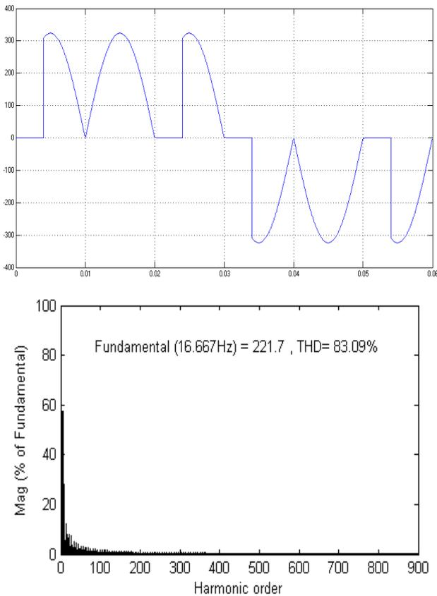
Fig. 11: Half Wave Symmetry Variable Firing Angle Method
