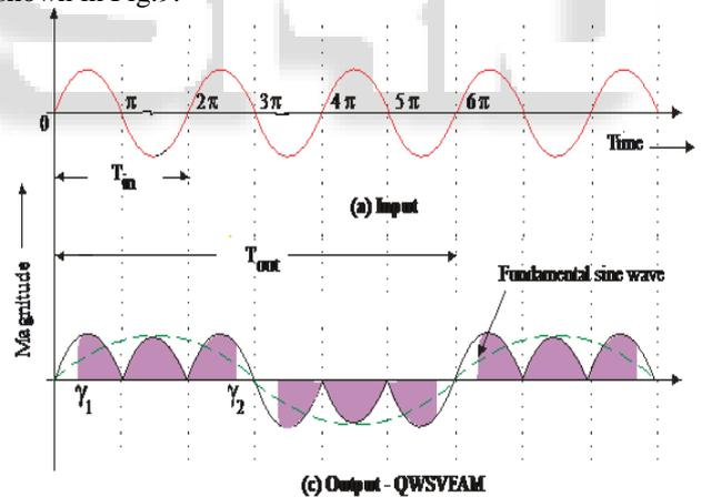
Fig. 9: Quarter wave symmetry variable firing angle method
