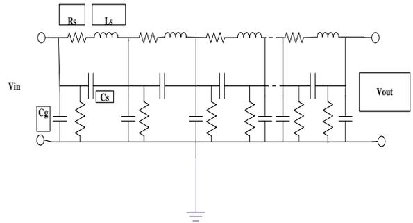
Fig. 3: Transformer winding parameters
