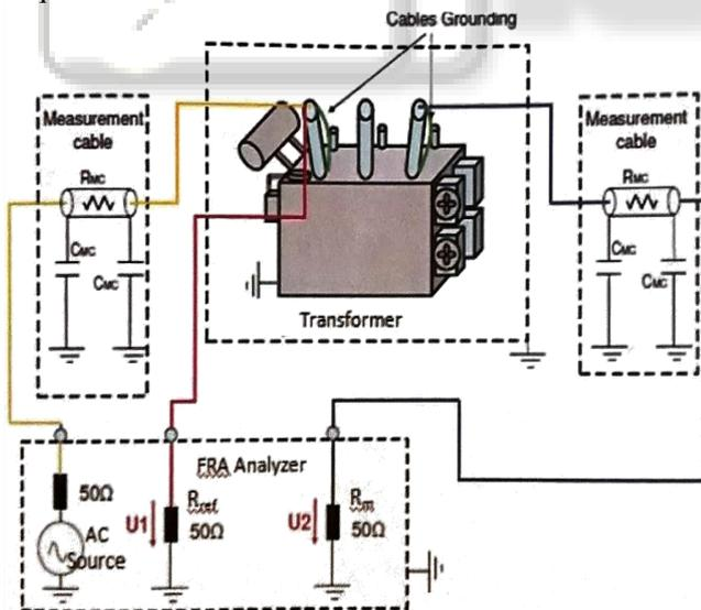
Fig. 1: SFRA measurement layout
