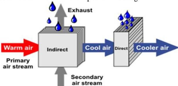
Fig. 4: Indirect/Direct Evaporative Cooling
