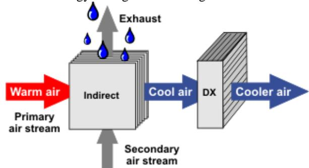
Fig. 5: Indirect evaporative cooling/DX
