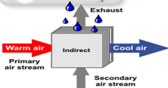
Fig. 3: Indirect evaporative cooling system
