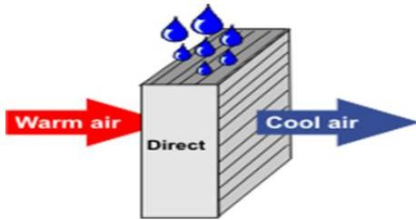
Fig. 2: Direct Evaporative Cooling System
