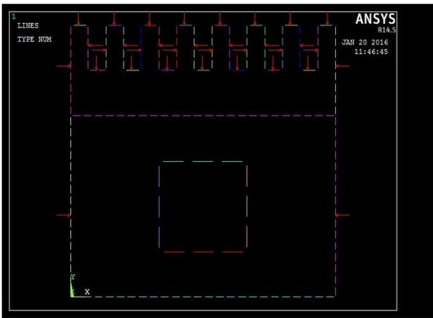
Fig. 2: Convective boundary condition on the walls
