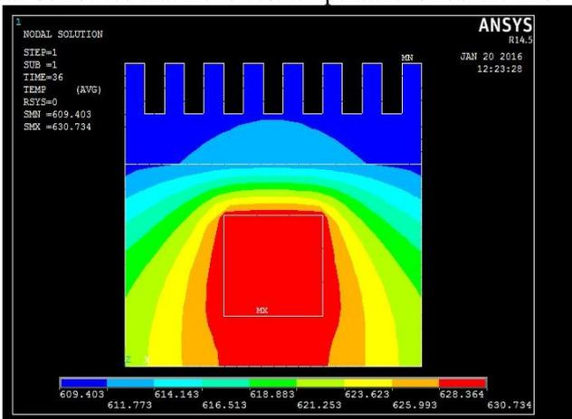
Fig. 3: Temperature distribution in the electronic device
