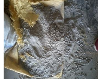
Fig. 4: Separated mortar after sieving
