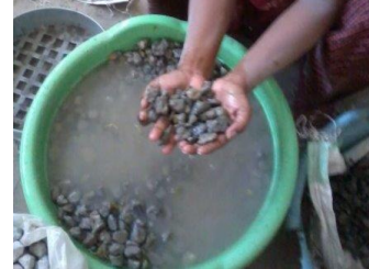
Fig. 5: Soaking of recycled aggregates
