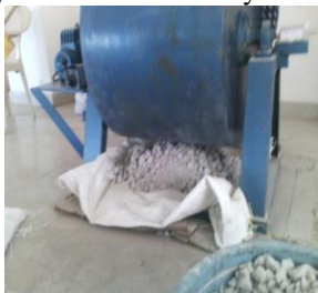
Fig. 2: Separation of mortar by using Los Angeles Abrasion Machine.
