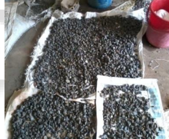
Fig. 6: Surface drying of RCA
