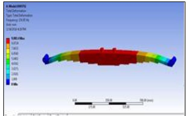
Fig. 4: Mode1 natural frequency of component with 6% of silicon nitride.
