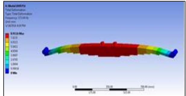
Fig. 5: Mode1 natural frequency of component with 10% of silicon nitride.
