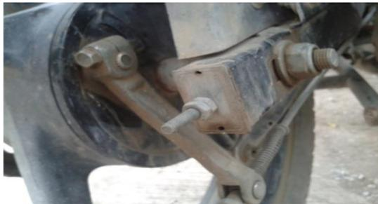
Fig 1: Chain Adjuster Bracket
