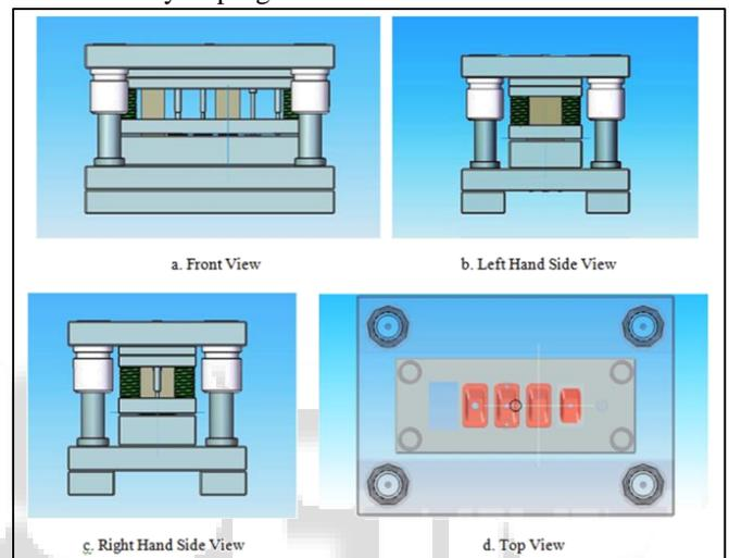
Fig. 3: Assembly and various views of progressive die set
