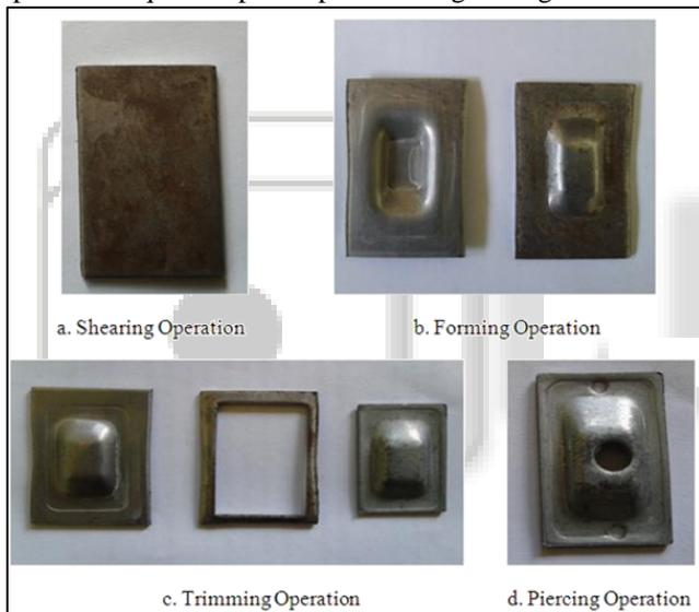
Fig. 2: Actual Processes for production of chain adjuster bracket
