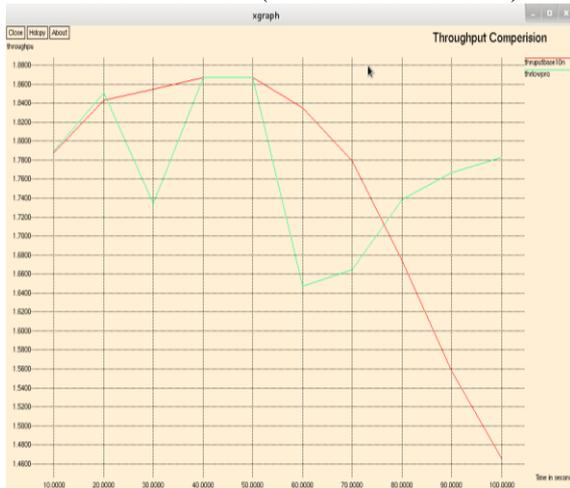
Fig .7: Throughput graph for low environment (10 nodes)
