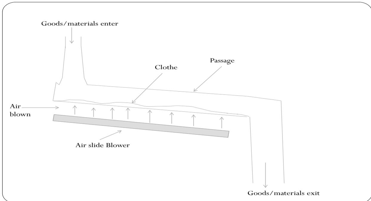
Fig. 2.1: Raw mill separator air slide.
