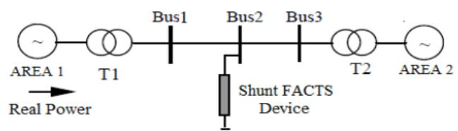
Fig. 1: Two-Area Power System with FACTS Device.
