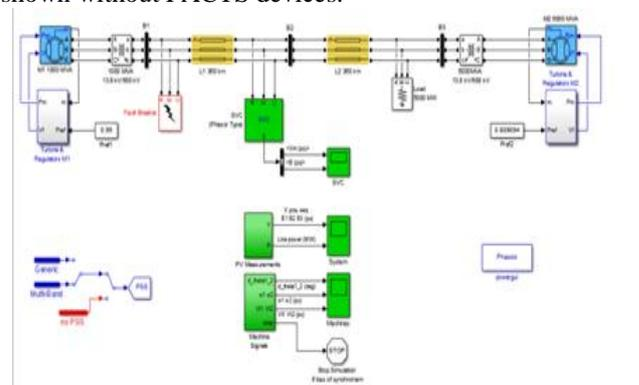
Fig. 3: Two Machine Power System Simulink Model with SVC Controller
