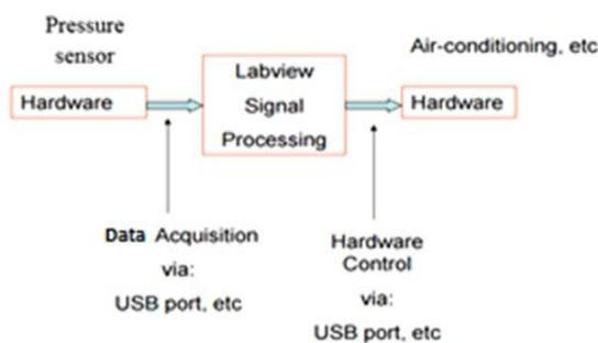
Fig. 2: A Schematic diagram of an instrument system based on LabVIEW.
