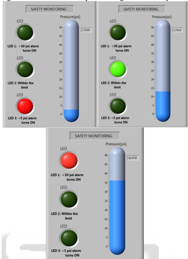
Fig. 8: Front panel design for safety monitoring of pressure process.
