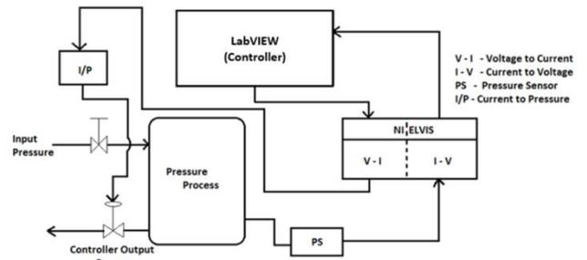
Fig. 4: Schematic diagram of pressure process in ELVIS interface.
