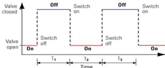
Fig 6: On-Off control graphical representation of pneumatic actuator
