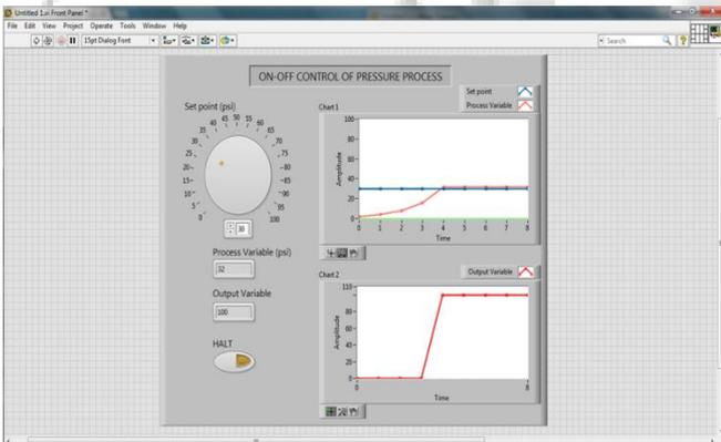
Fig 7: Front panel design for On-Off control action of pressure process
