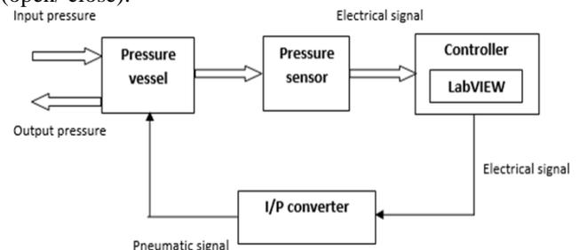
Fig. 1: Block diagram of complete pressure process.
