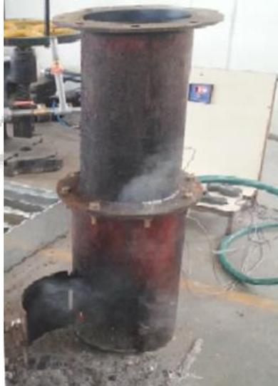
Fig. 1: Photograph of Downdraft Gasifier
