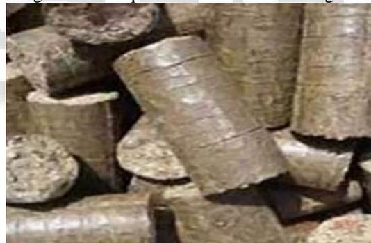
Fig. 3: Sugarcane Briquette Sample Used for Experiment
