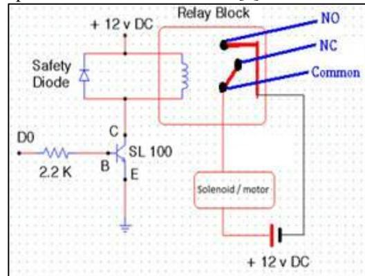
Fig. 7: Relay circuit [2]
