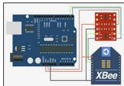
Fig. 9: Arduino Xbee Wireless Modem [10]
