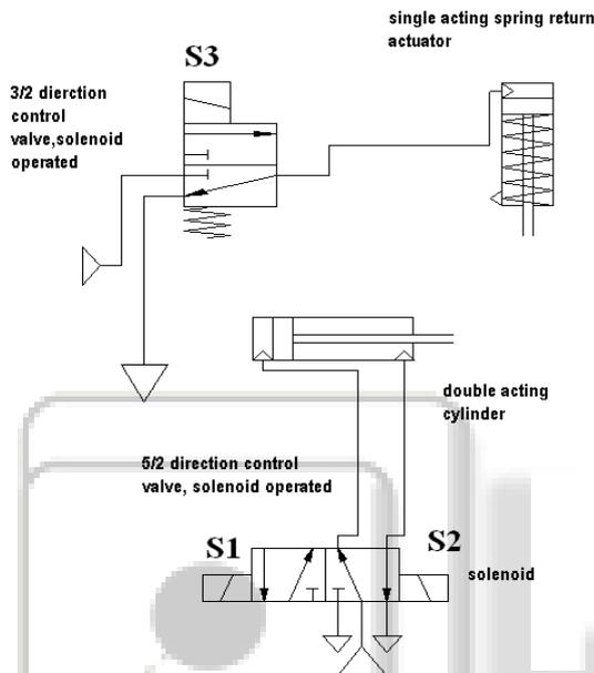
Fig. 5: ElectroPneumatic circuit using Automsim Premium [9]
