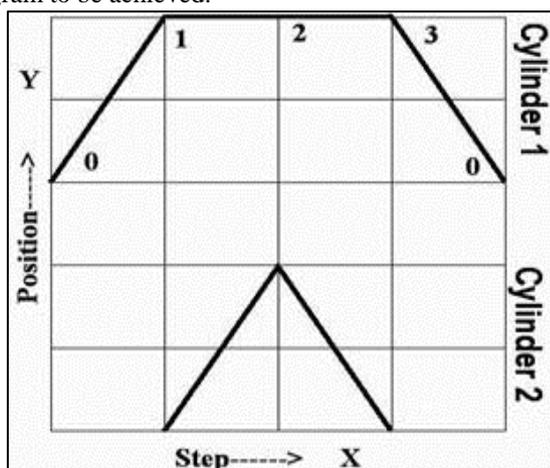
Fig. 6: Position Step diagram [9]
