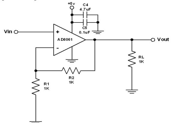
Fig. 4: Serial Buffer circuit [14]
