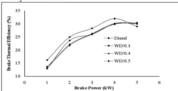
Fig. 1: Brake Thermal efficiency Vs Brake power.
