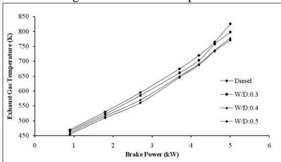
Fig. 6: Exhaust Gas Temperature vs Brake power.
