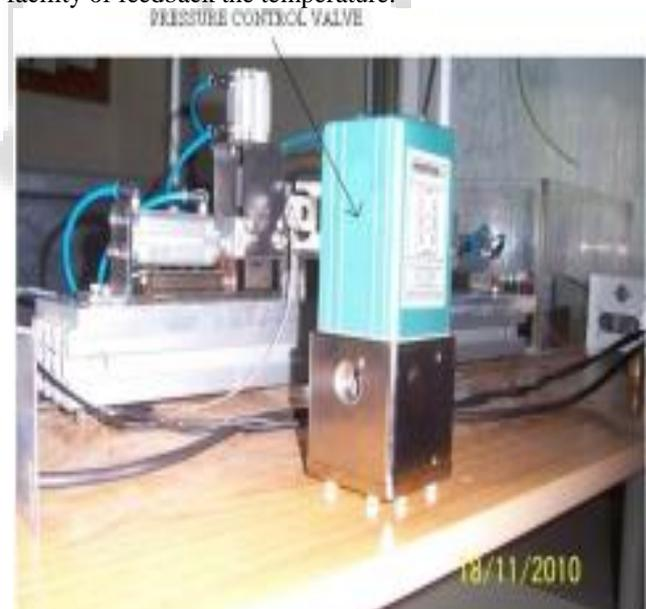
Fig. 6. Pressure Control Valve.
