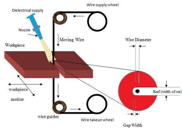
Fig .1: Working principle of WEDM
