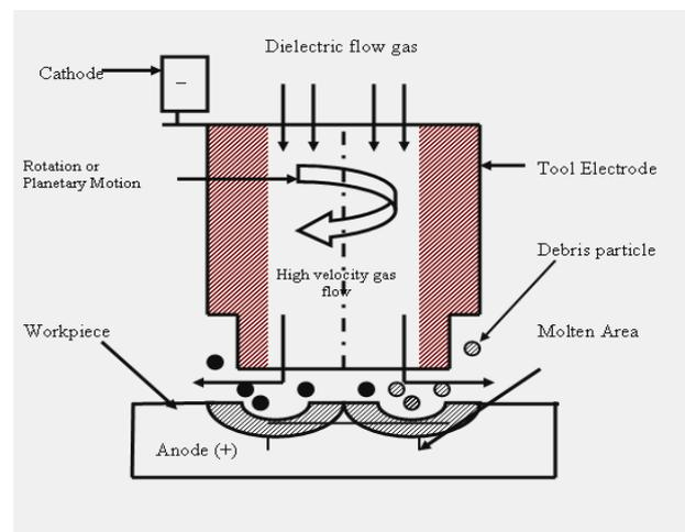
Fig. 2: principle of dry wire EDM
