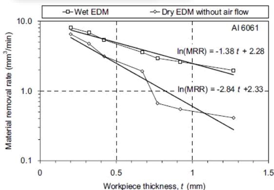
Fig. 3: Effect of thickness on MRR of AL 6061 for wet and dry EDM.
