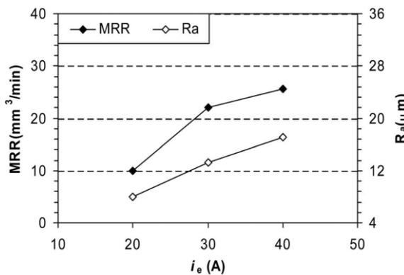
Fig. 4: Effect of the discharge current on high energy input dry EDM with
