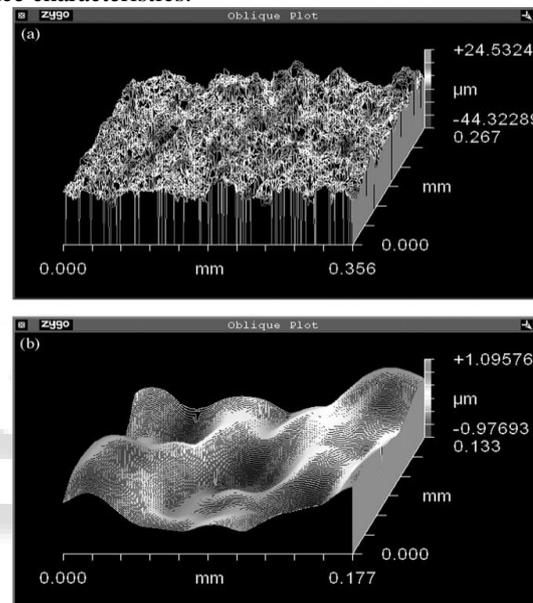
Fig. 4: (a) Optical profile of a surface machined using WEDM with surface roughness 3.06μm Ra.
