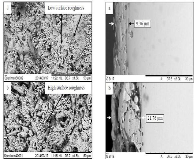
Fig. SEM micrograph at different levels of spark energy. a) SEM micrograph at the lowest levels of peak current (IP=1.6A) and pulse on time (Ton=0.15µs). b) SEM micrograph at the highest levels of peak current (IP=1.7A) and pulse on time (Ton=0.25µs)
