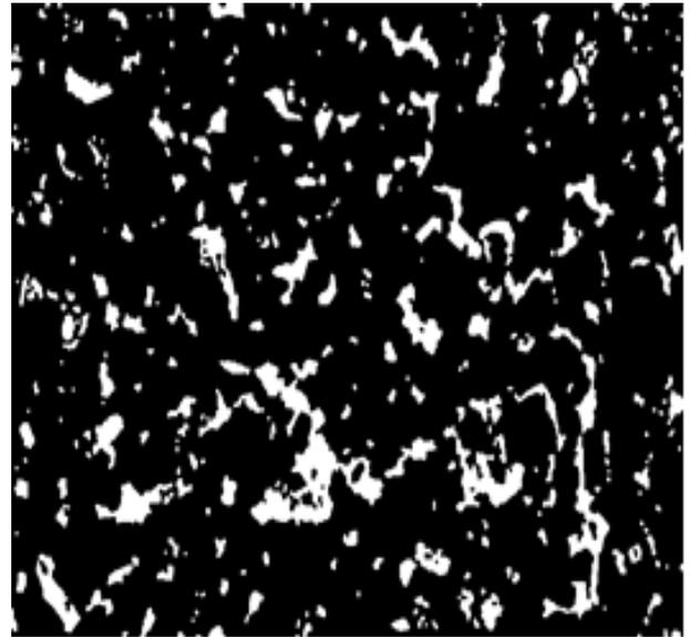
Fig. 9: Binarization of sandstone sample.
