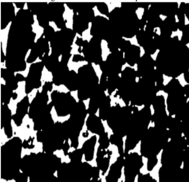
Fig. 8: Binarization of sandstone sample.
