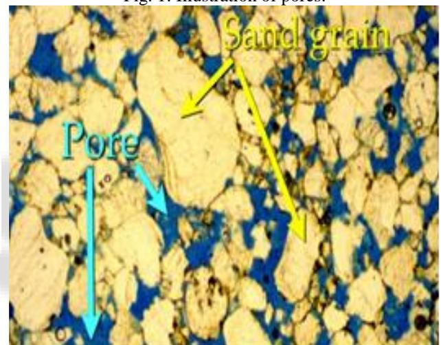
Fig. 2: Illustration of pores for thin section of a sandstone rock.
