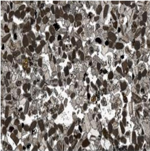
Fig. 6: Sandstone rock sample.
