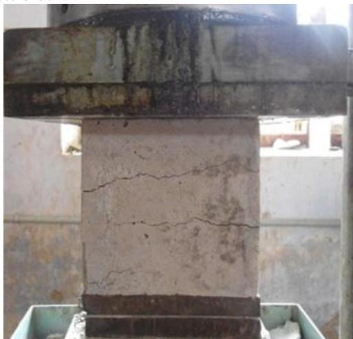
Fig. 4: Hairline Cracks in Concrete Block
