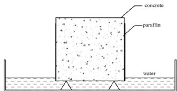
Fig. 5: Capillary Absorption Equipment Setup
