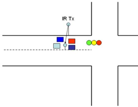
Fig. 4: IR Rays out of Range of Vehicle
