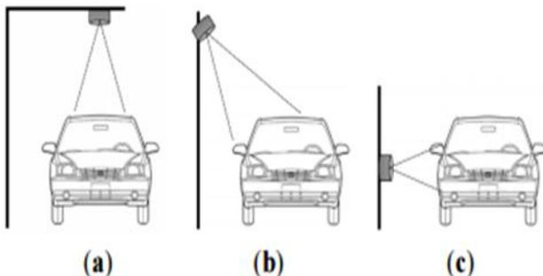
Fig. 2. Ultrasonic Sensors for Traffic Control System
