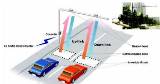
Fig. 1: IR sensors for Traffic Control System
