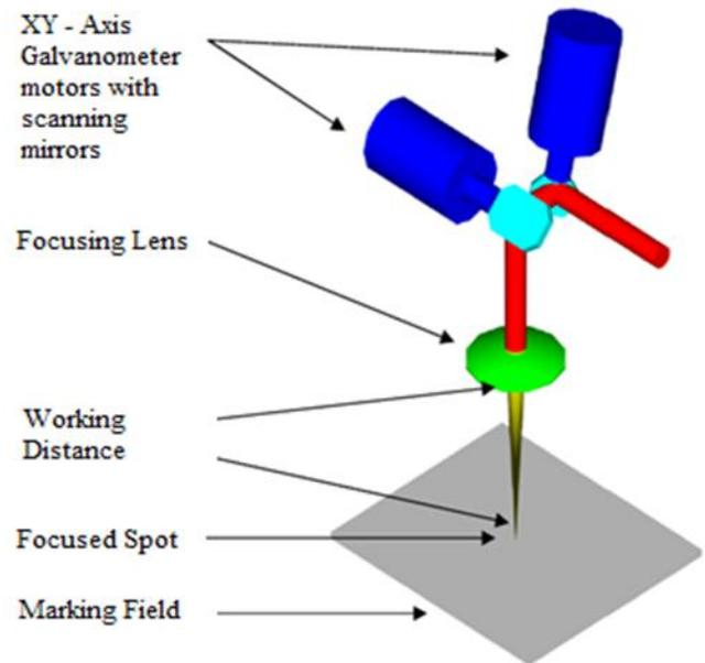
Fig. 1: Laser Engraving Process Setup
