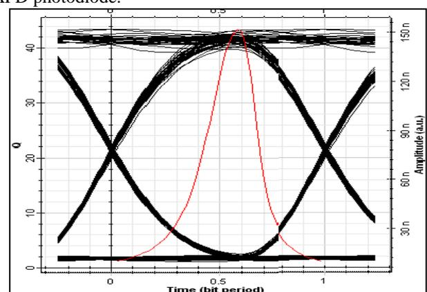
Fig. 2.2: Eye diagram NRZ modulated using APD photodiode system
