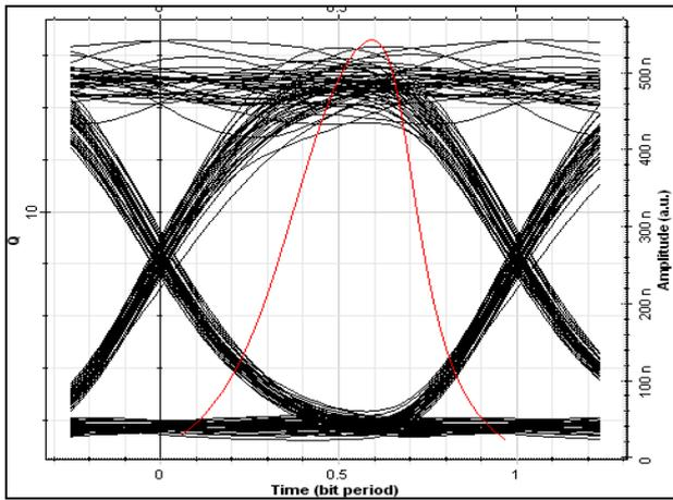
Fig. 2.3: Eye diagram NRZ modulated using PIN photodiode system
