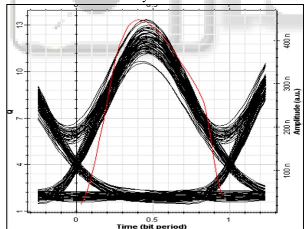
Fig. 2.5: Eye diagram RZ modulated using PIN photodiode system
