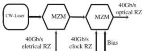
Fig. 3.1: Block diagram of RZ
