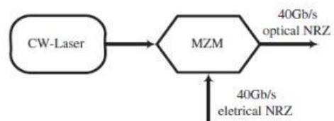
Fig. 3.1: Block diagram of NRZ
