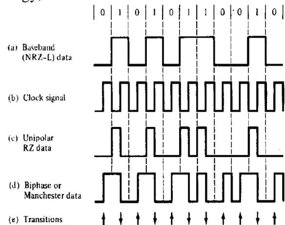
Fig. 2.1: Different coding techniques
