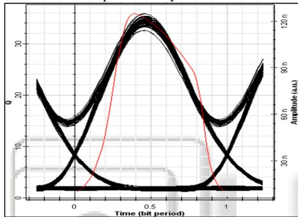
Fig. 2.4: Eye diagram RZ modulated using APD photodiode system
