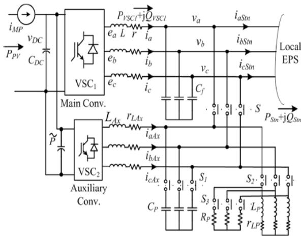
Fig. 1: Proposed power circuit of PV-DGS with auxiliary converter and RPB.
