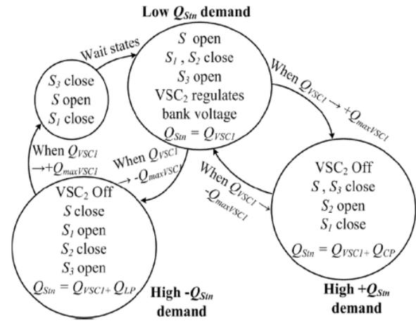
Fig. 2: State machine diagram of the proposed re-active power enhancement scheme.
