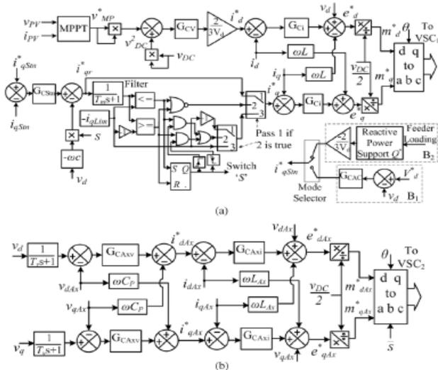
Fig. 7: Control scheme for the proposed reactive power enhancement system with only capacitor bank and switch in operation. (a) Control. (b) Control.
