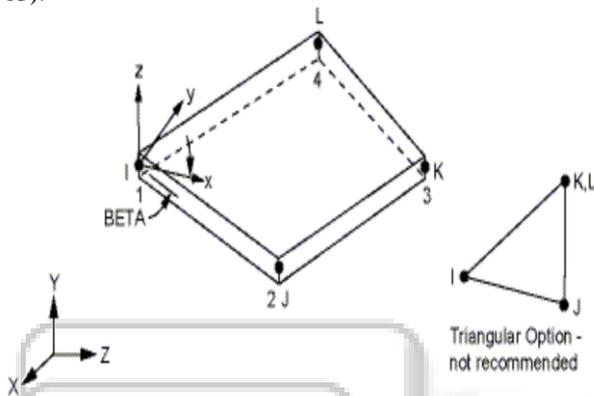
Fig. 1: Shell 163, 4-Noded Quadrilateral Shell Element. SHELL163 is a 4-node element with both bending and membrane capabilities as shown in figure 1. Both in-plane and normal loads are permitted. The element has 12 degrees of freedom at each node: translations, accelerations, and velocities in the nodal x, y, and z directions and rotations about the nodal x, y, and z-axes
