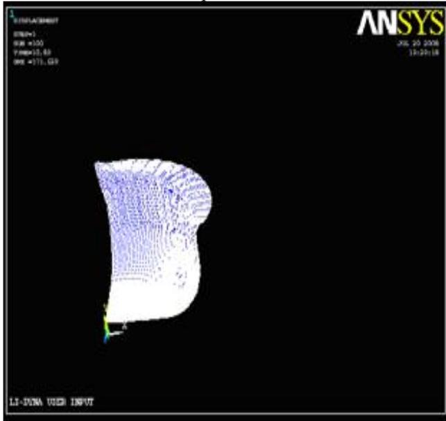
Fig. 4: Product Showing Wrinkle at Coefficient of Friction 0.2.
