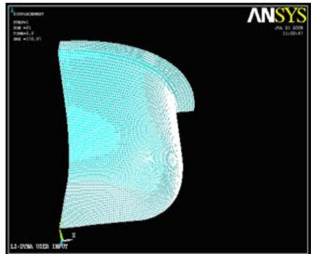
Fig. 5: Wrinkle Free Product at Coefficient of Friction 0.25
