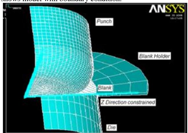
Fig. 3: Model with Boundary Condition.
