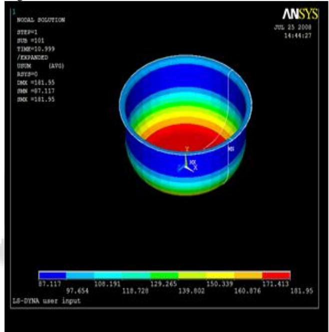
Fig. 6: Full Model of Deep Drawing at End of the Stroke.
