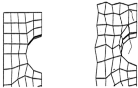
Fig. 2: Unreformed Mesh and Deformed Mesh with Hour Glassing Effect.
