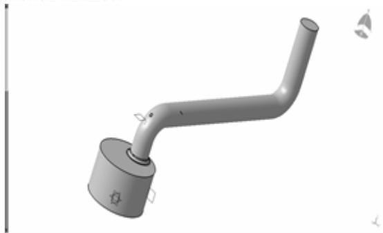
Fig. 2: Swirl Enhancing Device with Inlet Manifold
