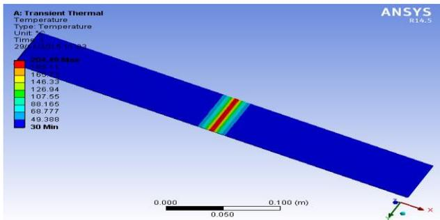
Fig. 6: Temperature distribution in welding plate by FEM
