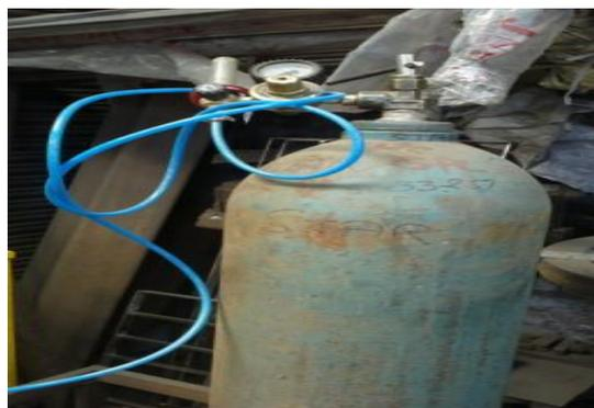
Fig.1. (b) Argon gas cylinder
