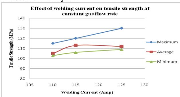
Fig. 9: Welding current vs. Tensile strength
