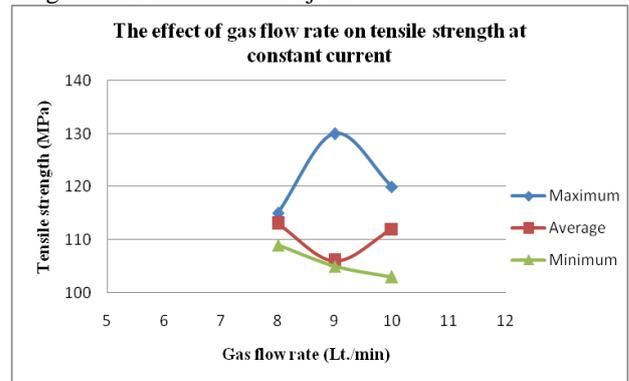
Fig. 10: Gas flow rate vs. Tensile strength
