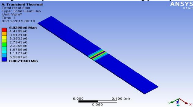
Fig. 7: Heat Flux in welding plate by FEM
