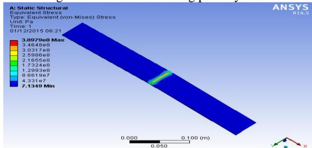
Fig. 8: Stress distribution in welding plate by FEM
