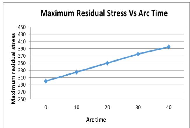
Fig. 16: Maximum residual stress vs. Arc time
