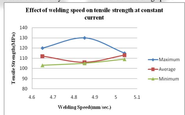
Fig. 11: Welding speed vs. Tensile strength
