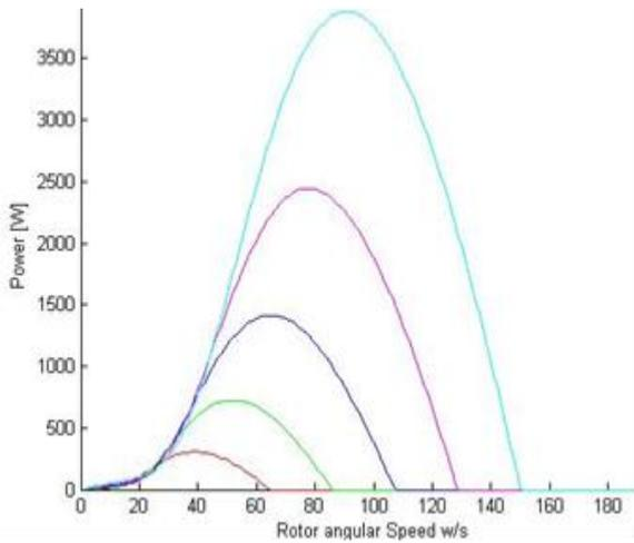
Fig. 3: Power speed characteristics of WTG
