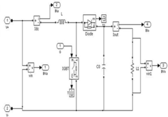
Fig. 4: Simulink diagram of Boost converter.
