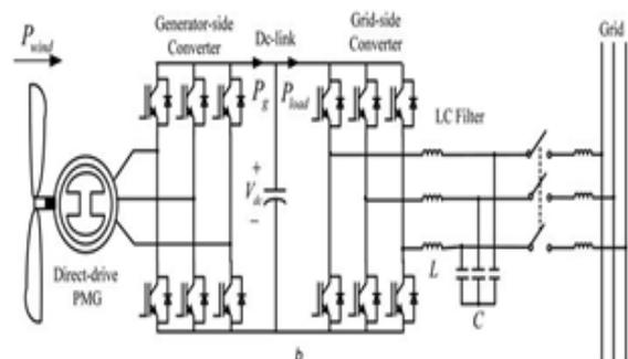
Fig. 2: WTG with PMSG.
