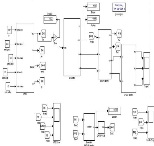
Fig. 6: Simulink model of Wind turbine generator.
