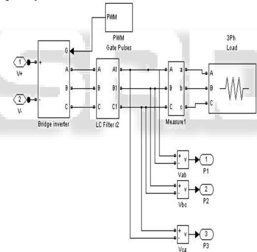
Fig. 5: Simulink model of Inverter.
