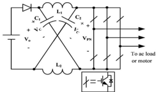
Fig. 1: Z-source Inverter
