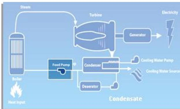
Fig. 1: Typical power plant layout
