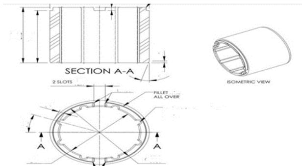
Fig. 6: Ketron Peek Metal Bearing
