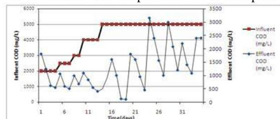
Fig. 4: Influent COD and effluent COD during the treatment range (29°C to 37°C) during the study. The increments in feed concentrations were made in steps at a HRT of 12 hours until the confirmation of granulation. Feed concentration was increased from 2000 mg/L to 4000 mg/L.
