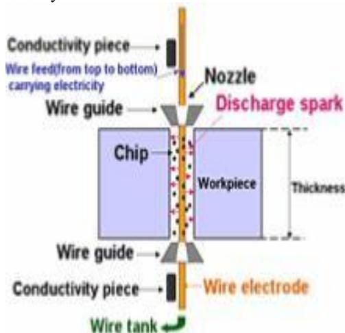
Fig. 1: Mechanism of material removal of WEDM [1]
