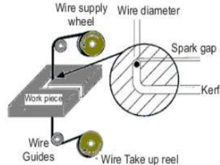
Fig. 2: Details of WEDM gap [2]
