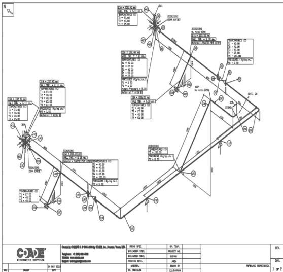
Fig. 2: Stress isometrics for pump suction sheet 1 of 2
