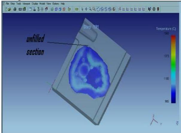
Fig. 1: Simulation of End Plate at 1000 oC
