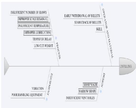
Fig. 7: Cause and Effect Diagram for Unfilling
