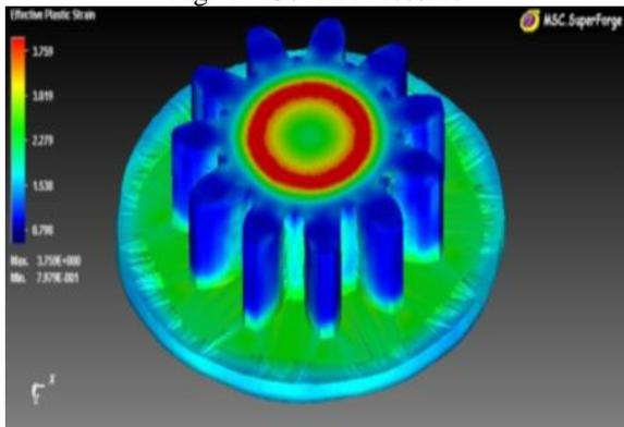
Fig. 3: Effective Plastic Strain
