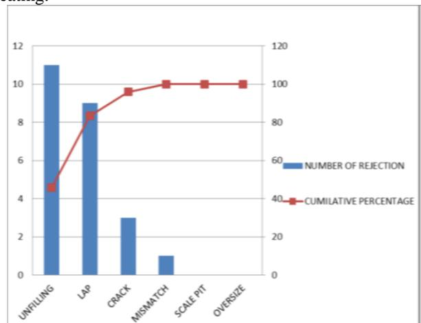
Fig. 6: Defect Analysis Using Pareto Diagram
