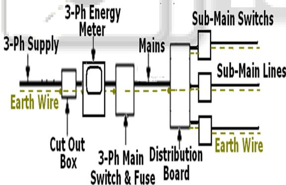
Fig. 7: Schematic Diagram Of Domestic 3-Phase Power Supply
