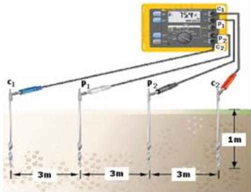
Fig. 6: Arrangement of Soil Resistivity test by Meter
