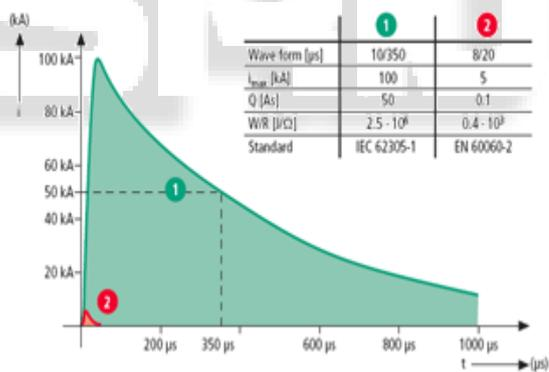
Fig. 9: Lightning and Surge Voltage Curve or Impulse Voltage Curve
