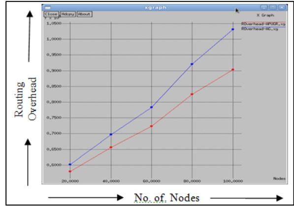
Fig. 4: Routing overhead Vs No. of Nodes
