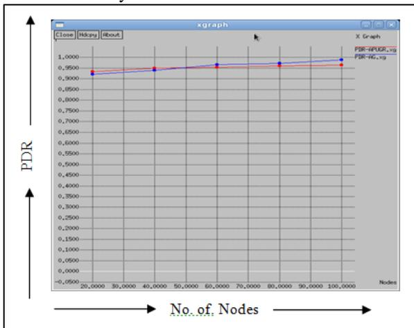
Fig. 3: Packet Deliver Ratio Vs No. of Nodes
