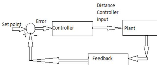
Fig. 1: structure of PID controller
